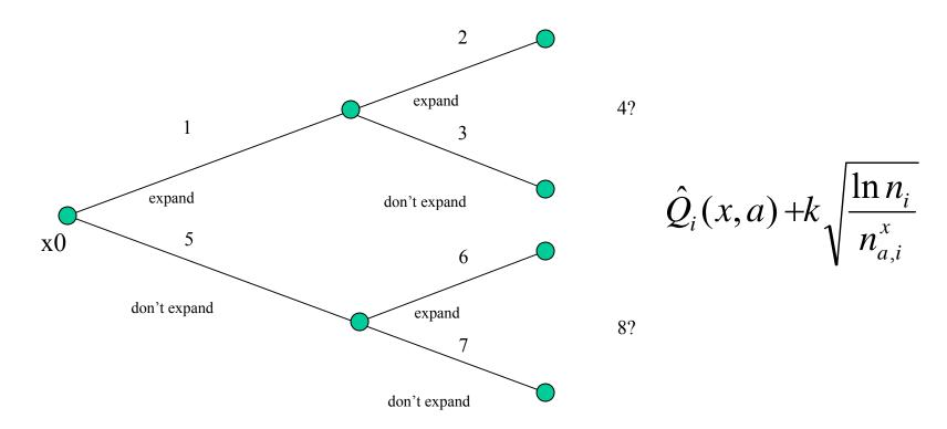
Nodes represent simulated state reached from simulation, numbers indicate sequence of simulations carried out
